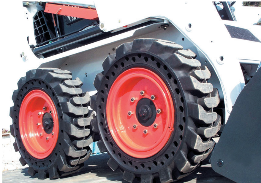
Solid tyres with sidewall apertures for shock absorption.
