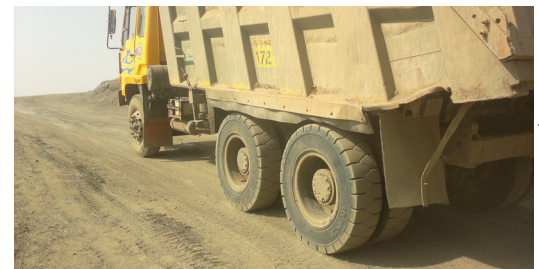
Tipper using solid tyres in a stone quarry.
